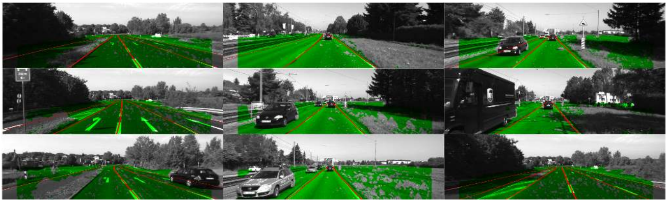
Fig. 7. Experimental results. The regions in green are estimated road surface areas. The lines in red are detected lanes.
